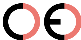
False CE Mark (too far)
